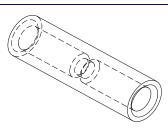
These solder sleeves provide a convenient method for making in line splices for attaching wires to feedthru, header or connector pins. They are self fixturing on the pin and both the wire and the pin solder joints are made in a single solder operation (refer to page 2 for application sequence). Shrink sleeving can then be slid into place and shrunk to prevent pin to pin shorts.
